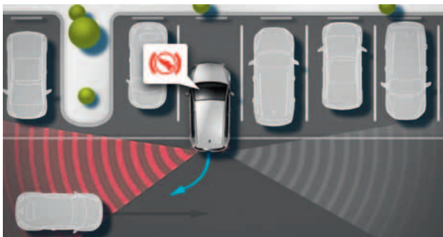
The Rear Traffic Alert alerts the driver to traffic that might not be visible to him. If the driver does not react to this, it can initiate emergency braking.
